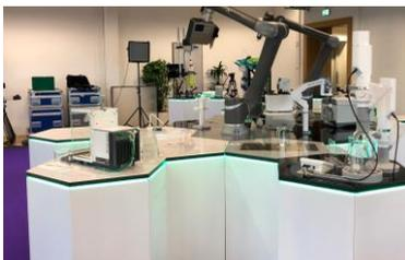
The honeycomb-shaped modules of the iHex laboratory system can be flexibly arranged and connected via plug-and-play to form a complete system
